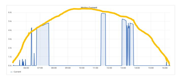
This figure shows the pump motor current trend over one day, which is representing most of the days. The graph shows that the pump is irregularly running. Depending on the irradiation, the pump power is regulated accordingly. Significantly more pumping capacity would be possible, so that more water could be supplied overall. An increase in the water storage tank and adjusted times of use can already be sufficient to pump enough water.
