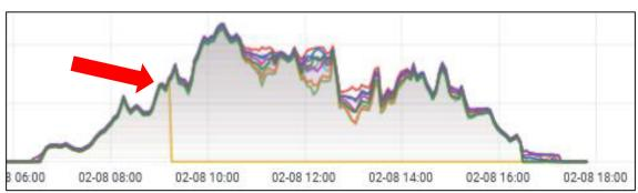
Both figures show the current of the respective strings of the solar system. The upper figure shows a regular pattern. The lower figure shows that the current of one string drops abruptly to zero.
